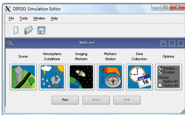
Figure 16-1 The DIRSIG Simulator Editor provides access to various components of the program.
