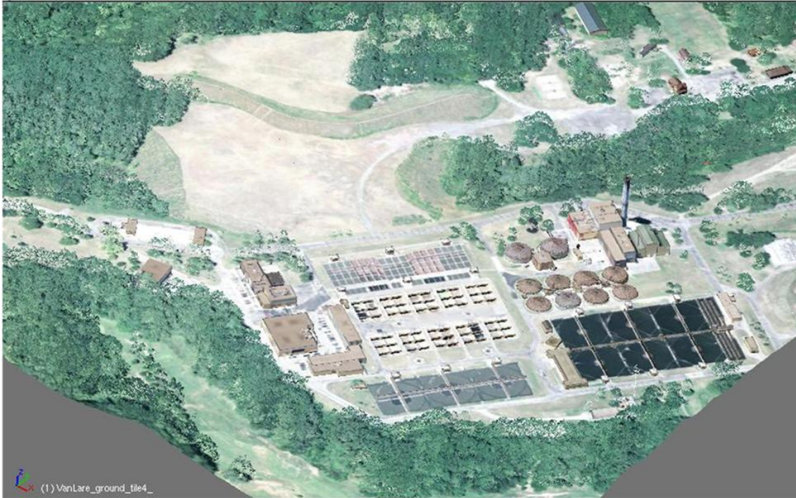
Figure 6-13 The final model of the VanLare site, as viewed in Blender, using manually derived multiview imagery building models (courtesy Pictometry Int.) and LIDAR derived terrain and tree models.
