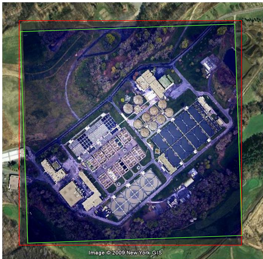
Figure 3-6 Comparison of Registered VNIR WASP image (outlined in green) overlaid on its initial location (outlined in red) with the detailed site model in GE.
