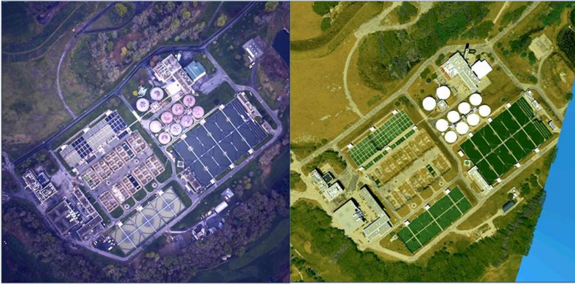
Figure 6-27 On the left is a contrast enhanced image of the VanLare plant taken by the WASP imaging system, while on the right, is similarly enhanced DIRSIG simulation of the same site using the WASP view and the Hybrid model of the site.
