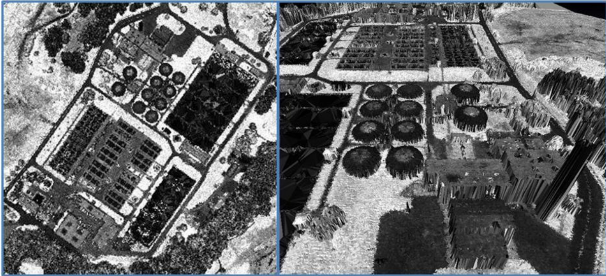
Figure 6-43 This figure shows the IR Attributed LIDAR model from a NADIR (right) and an oblique (left) view.
