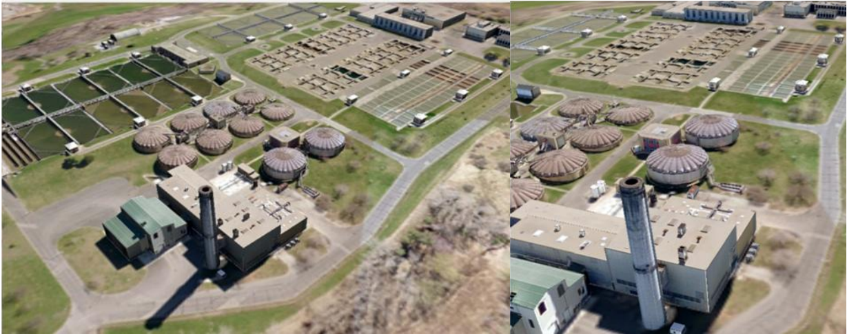
Figure 1-4 – The scenes above show the same model of the VanLare Plant from within the AANEE software program. Note the accurate casting of shadows and the ability to predict occlusions due to the 3D modeled site and landscape.
