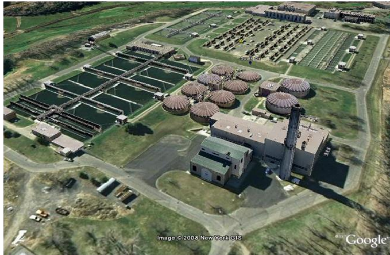
Figure 15-4 This realistic Pictometry model (Pictometry 2010) utilizes UV mapped oblique imagery to texture its facets and was then inserted into Google Earth (Google Earth 2010) using a KML description.
