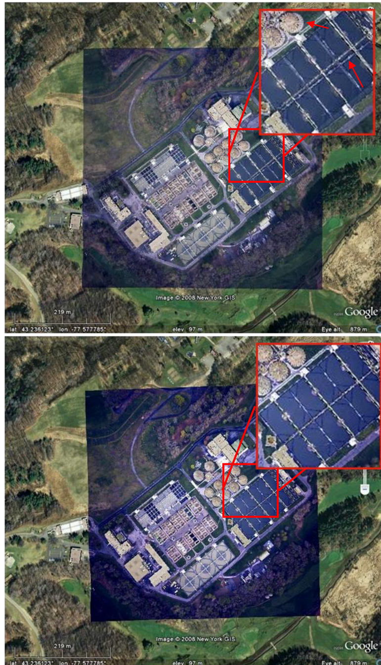
Figure 3-5 The top image with initial IMU/GPS pose and the bottom after affine correction. Both images are displayed in Google Earth with 30m accuracy terrain and detailed Pictometry model of the VanLare Site.
