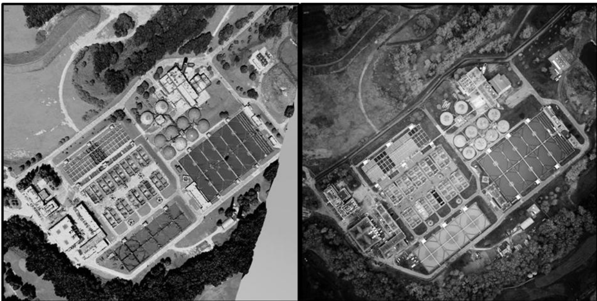
Figure 6-32 The LIDAR Direct DIRSIG simulation's similarity to real imagery is readily apparent. The ability to relate LIDAR derived models, textured with archival imagery, to newly acquired images is key to the model centric approach.
