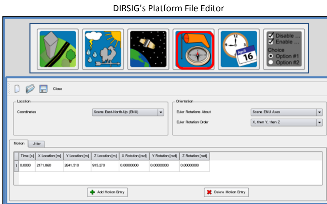
Figure 16-7 The Platform Editor allows for the designation of geospatial position information, such as Latitude, Longitude, Altitude and the orientation information of the sensors External Orientation Parameters, such as Pitch, Yaw & Roll.
