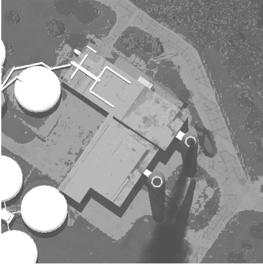
Figure 87: DIRSIG panchromatic image of a CH<sub>4</sub> gas plume inserted into the RIT's Megascene 1 water treatment facility
