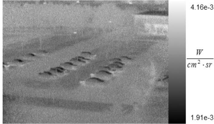
Figure 6.12: Example of surface leaving, aperture reaching radiance image, with polarizer at 0 degree orientation
